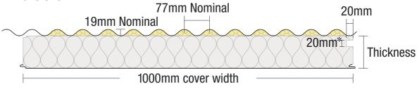
\* Services ducts 30x30mm are available for panel thicknesses 150-200mm
